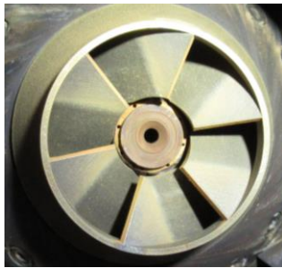
Figure 11: Additively manufactured burner head after the first minor hot gas path inspection.
