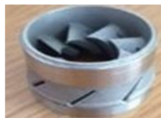
Figure 1: Advanced burner swirl manufactured by AM for SGT-750 industrial gas turbine
