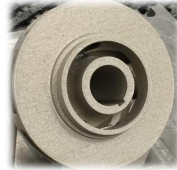
Figure 12: First 3D- printed impeller for a fire protection pump for the Krško nuclear power plant.
