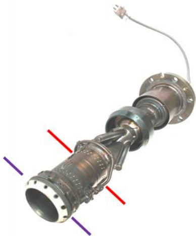
Figure 3: Gas turbine burner repairs in the traditional fashion (red line) and the described novel repair process (purple line).
