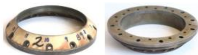
Figure 6: Burner tip area subject to destructive examination.
